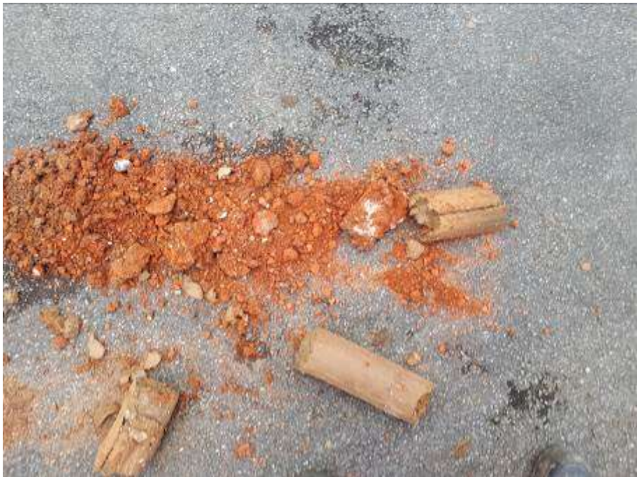
Plate 5 Showing arisings of crushed brick at WS03
