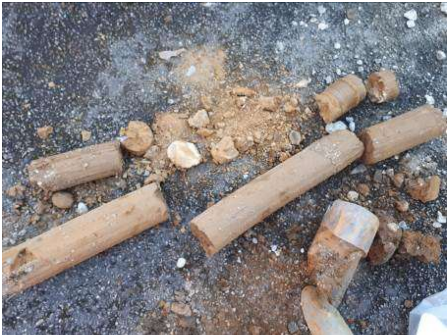
Plate 3 Showing the arising of clay within WS02 before backfilling the void
