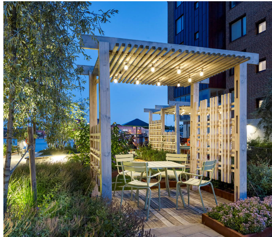
Lighting fixtures inside planters illuminate vegetation and catenary light illuminates the pergola
