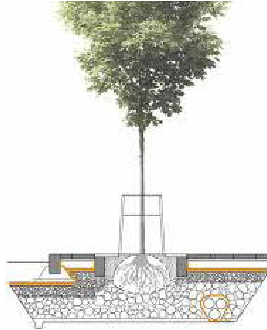
Structural soil ensures trees get the sufficient volume for their root system
