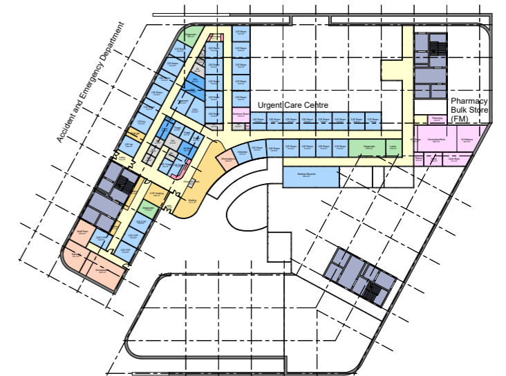
Test-to-fit layout for the A&E department, located on the lower ground floor
