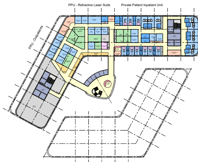
Test-to-fit layout for the private patients unit. At RIBA Stage 1 it was located on the seventh floor.
