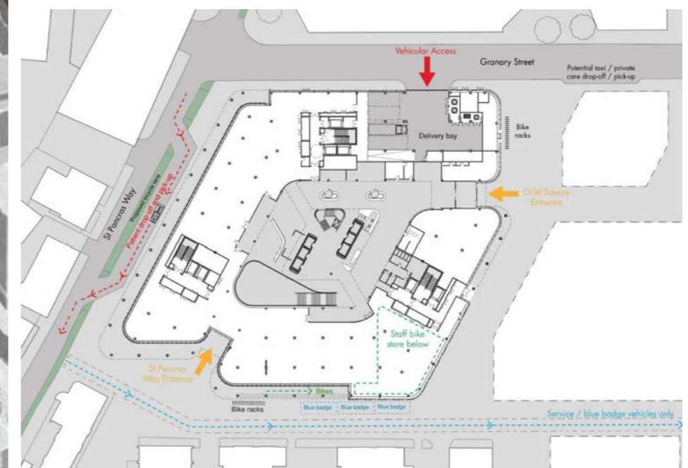
Final patient drop-off arrangement and building position
