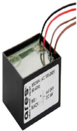
Code: 106 Supported n. of lamps: 1 Power supply dual function Vout 24Vdc: 8W/100÷240V Iout 350mA: 6X1W/100÷240V - IP65 CLASS II SELV EQ.
