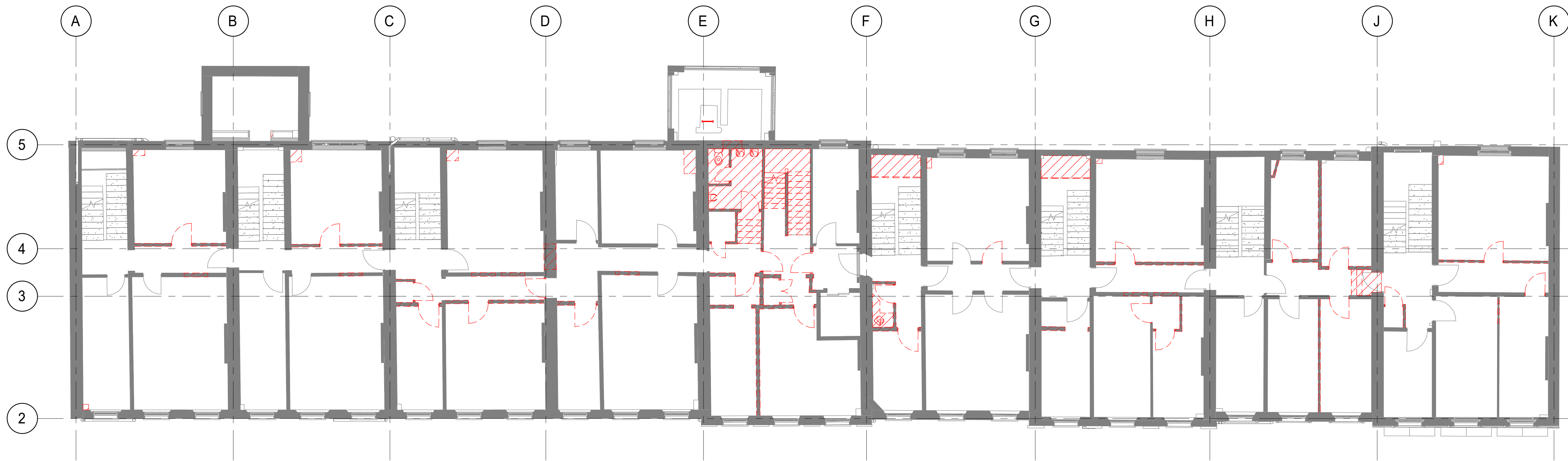
2. Planning - LEVEL 02 - Demolition Plan 1 : 100
