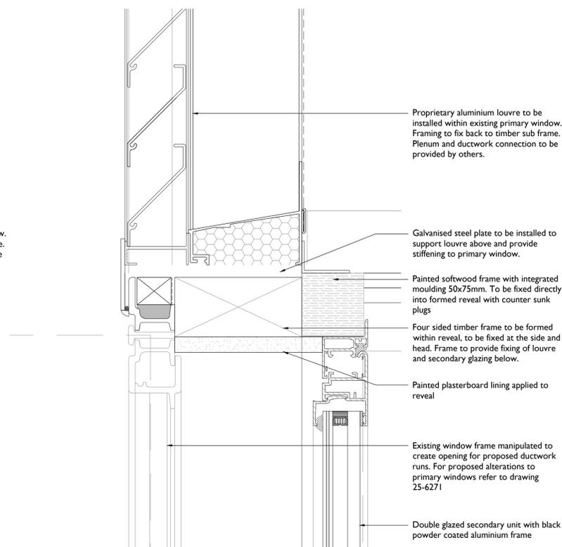
**8 Integrated louvre / Secondary glazing junction detail**
