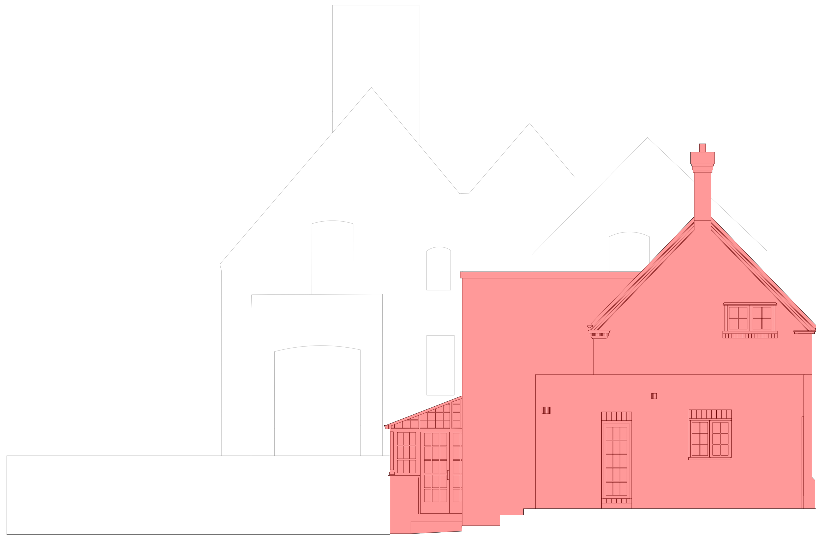
1 Demolition Side Elevation - East Scale: 1:50
