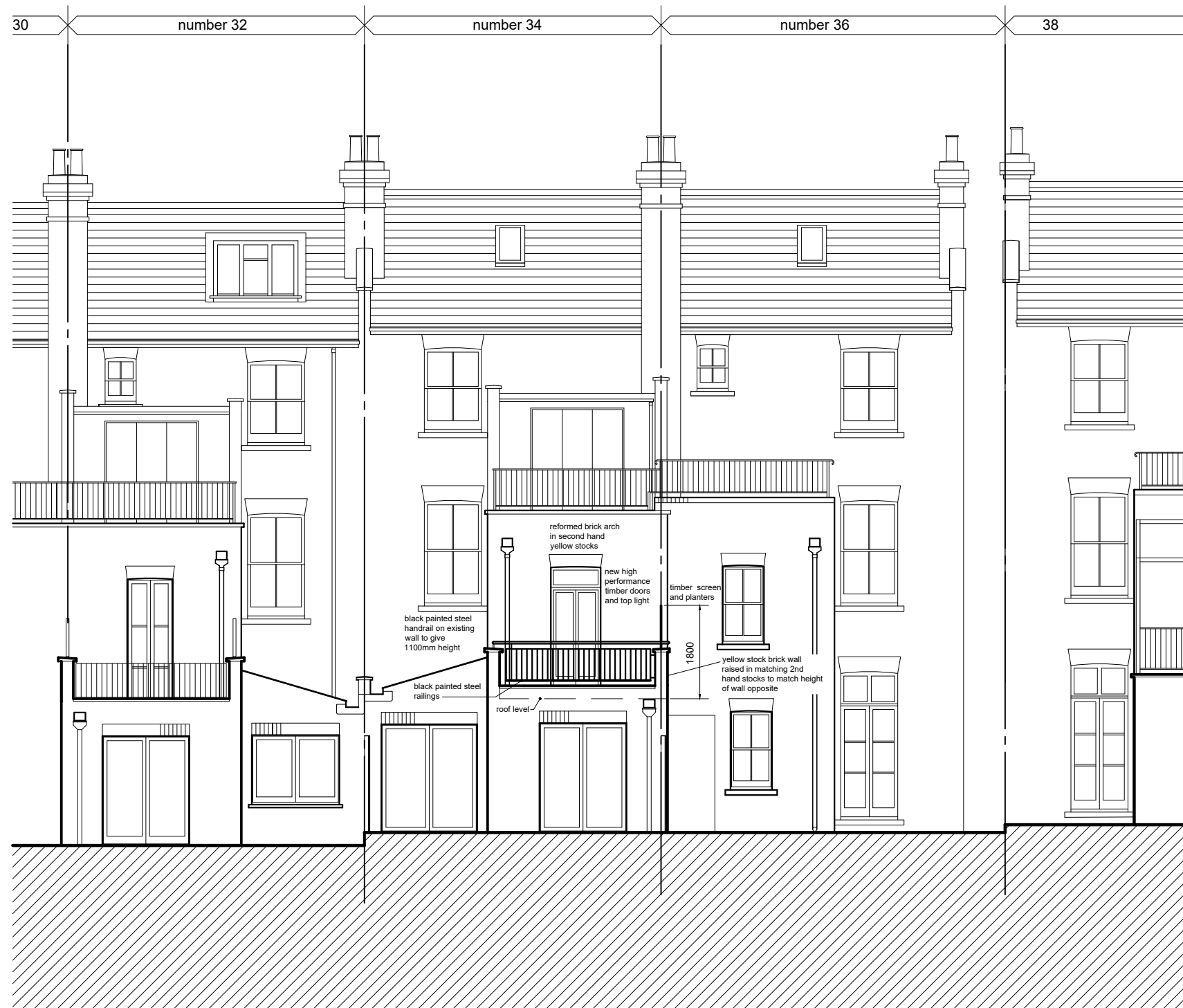
PROPOSED REAR ELEVATION OF NUMBER 34 SHIRLOCK ROAD INCLUDING NUMBERS 30,32,36 AND 38 SHIRLOCK ROAD
