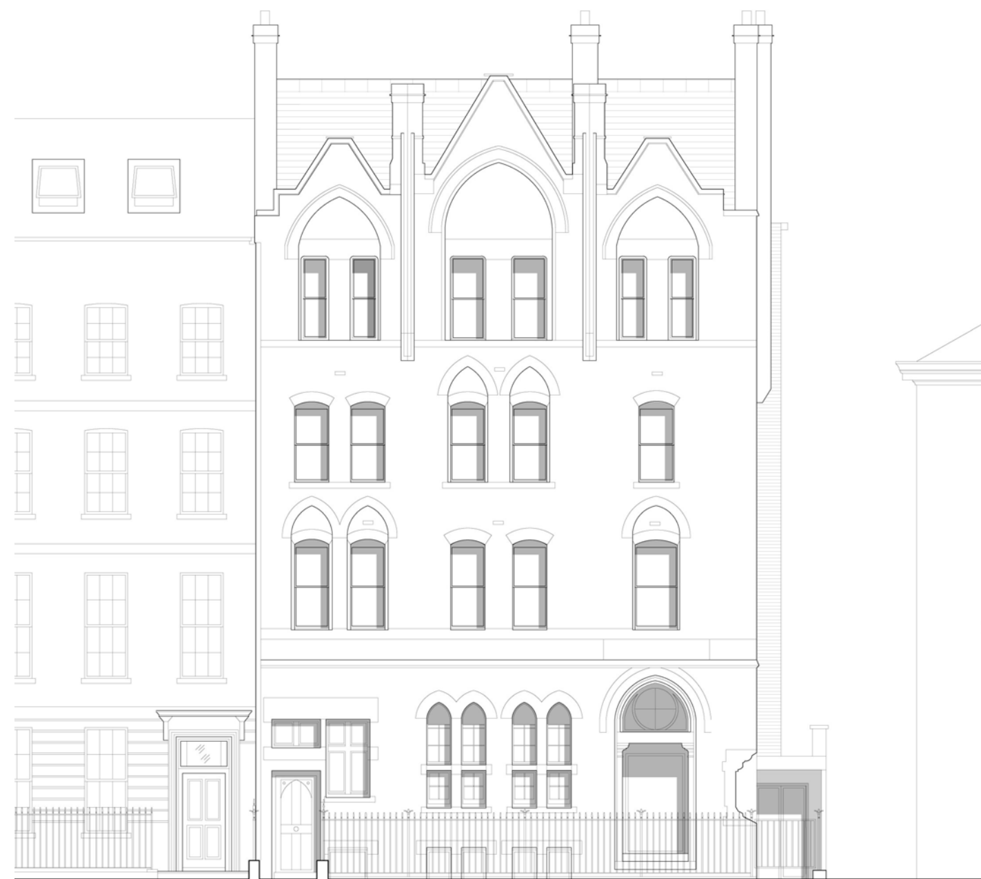
Proposed front elevation showing the proposed new side entrance to the D1 space on the right
