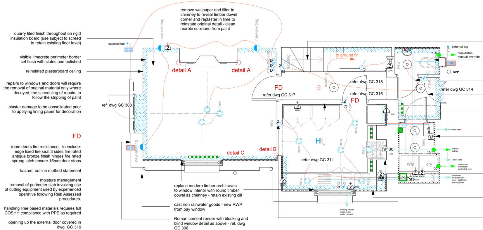
quarry tiled finish throughout on rigid insulation board (use subject to screed to retain existing floor level)
