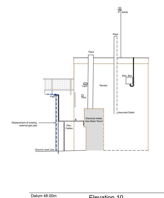
Datum 48.00m Elevation 10 (North Elevation)
