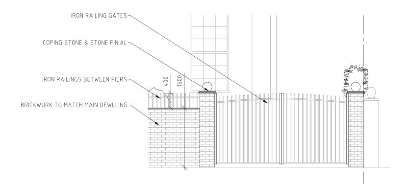
FRONT BOUNDARY WALL AS PROPOSED (EXTRACT) SCALE 1:50@A1
