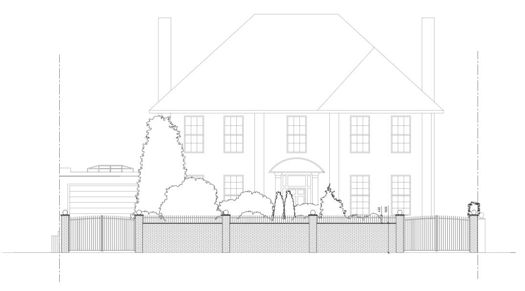
FRONT ELEVATION SHOWING PROPOSED FRONT BOUNDARY WALL SCALE 1:100@A1
