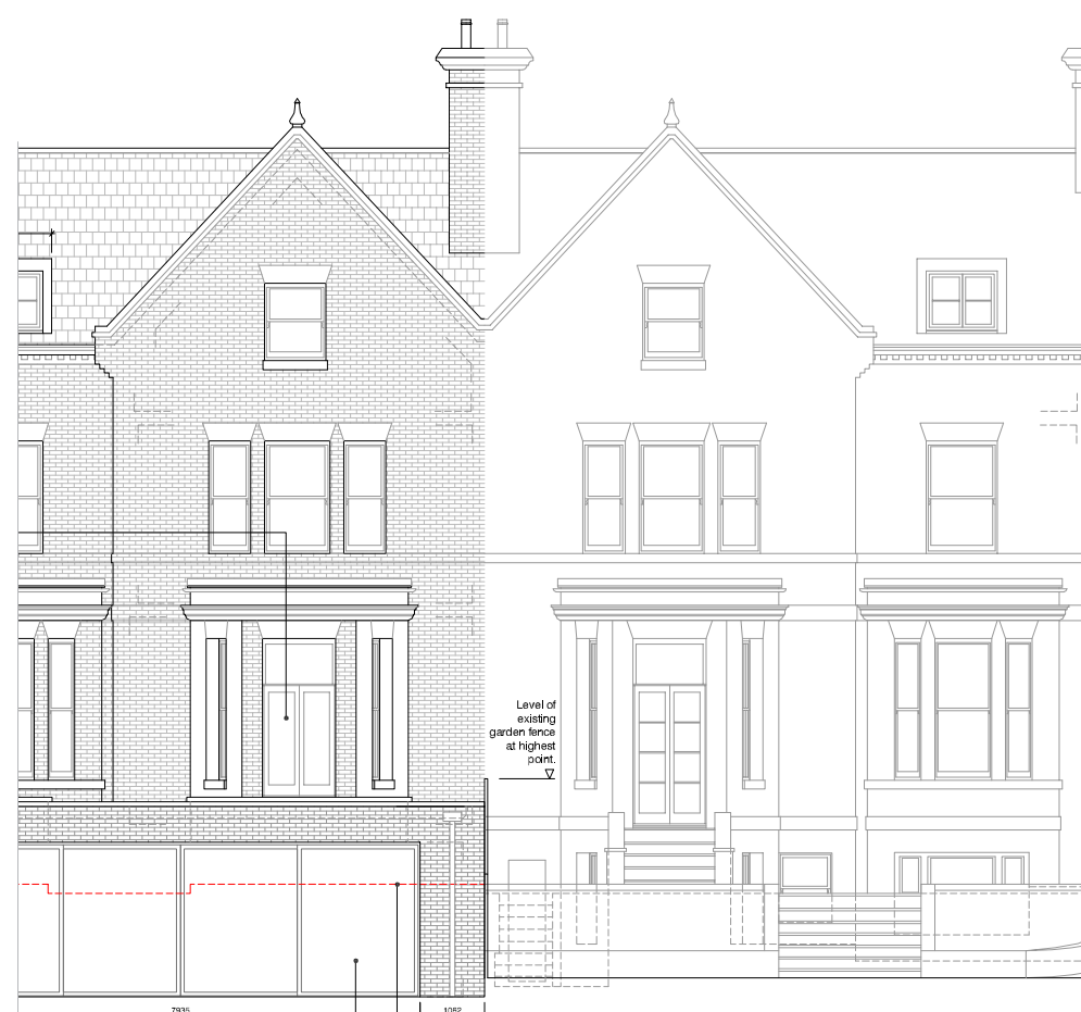
q) Rear elevations of no 18 and no 20 Hampstead Lane showing central access from main bay (from Haringey planning consent for no 10) and alignment of bay window openings
