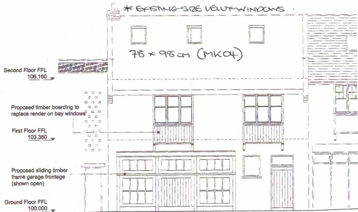
Front Elevation To 18 Deleham Mews (doors open)
