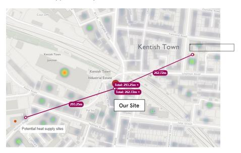
Considering the distribution would almost certainly need to avoid going under buildings, the distances would be even greater. Transferring heat over this distance wouldn't be efficient or financially favourable for the relatively small heating demand of these two new flats (flat 1 and 2). For the above reason connection to a district heating network has been ruled out as an option.
