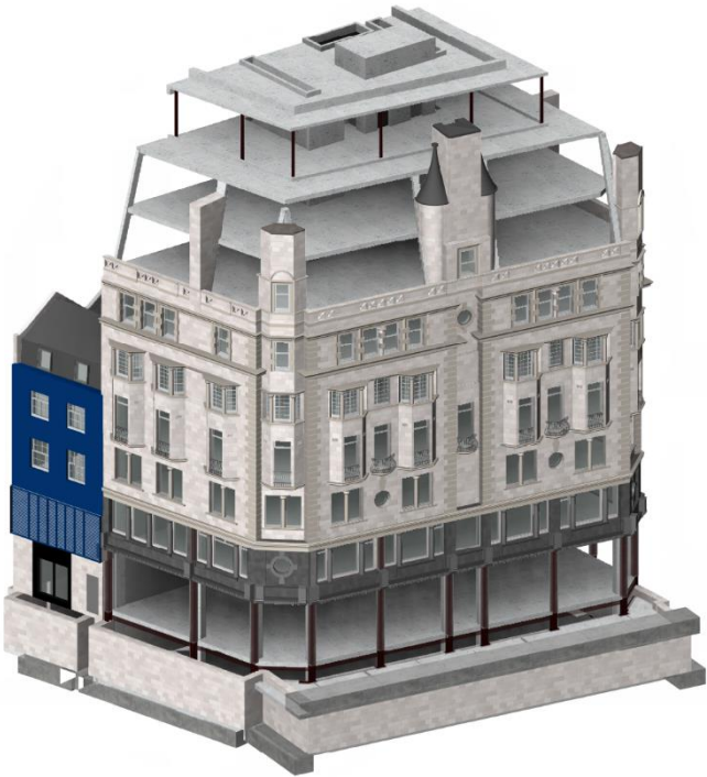
Completion of superstructure & removal of temporary works
