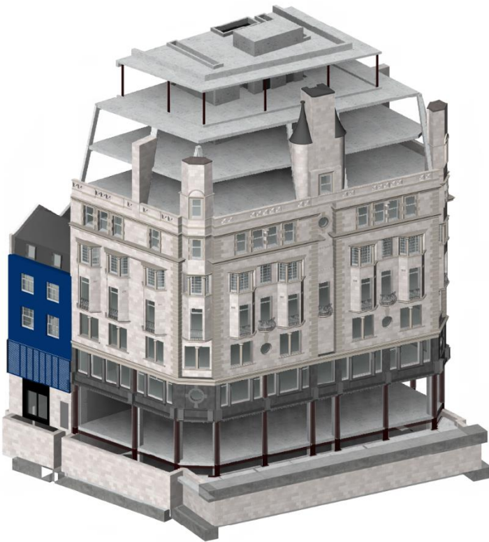
Figure 2.2: Existing Facade and Proposed Structural Frame
