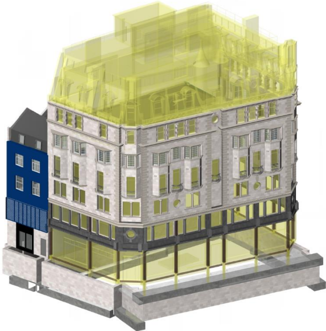
Demolition of mansard, internal structure and foundations
