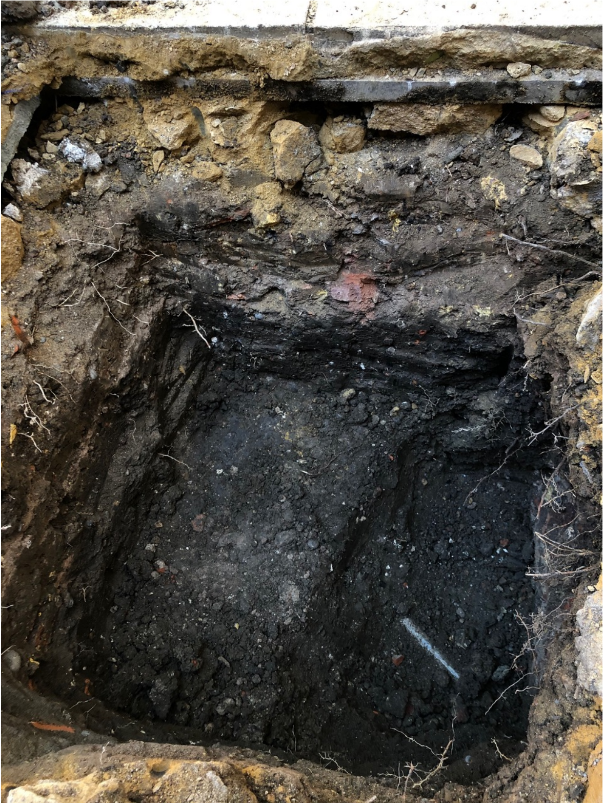
Photograph A2.2: Closer view of trial pit
