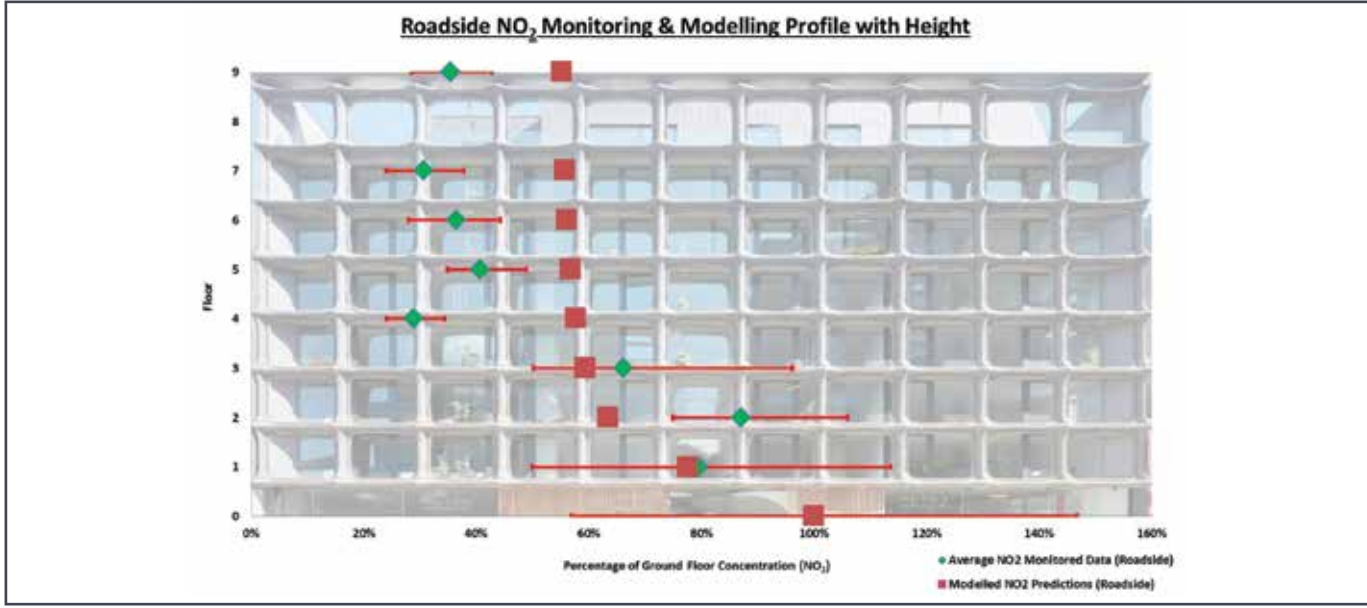
Figure 10: Comparison of roadside NO 2 diffusion tube monitoring and typical modelled concentration profile for NO 2 . The green points indicate the average monitored NO 2 concentration for each floor and the red bars indicate the minimum (left) and maximum (right) NO 2 concentrations measured at each floor. The red points indicate the modelled NO 2 concentrations predicted at each floor
