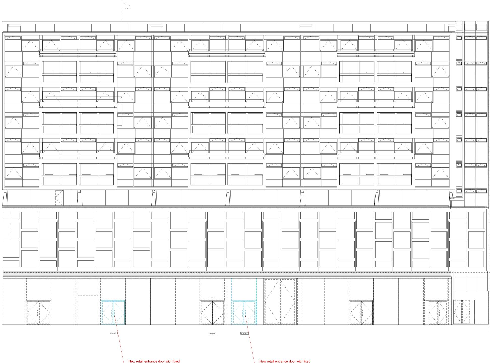
New retail entrance door with fixed glazed panel over to match existing doors (installed as part of refurbisment works).
