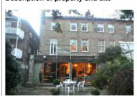
The subject property is a three storey semi-detached house which has been converted into three self contained flats. It is likely the property was built in around 1900 but the date of conversion is unknown. Construction is traditional with solid brick walls under a pitched slate roof. The property benefits from a single storey rear extension which is likely to have been built during the 1960's.
