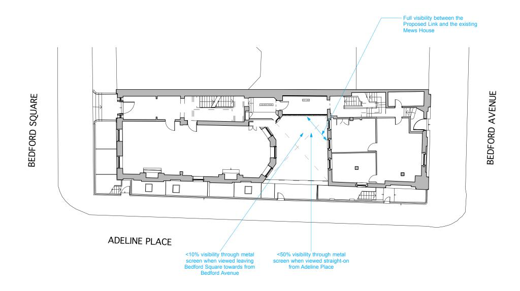
Proposed Ground Floor Plan - Visibility Diagram
