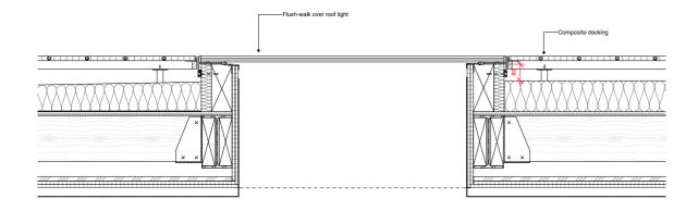
1 Flush Rooflight Detail
