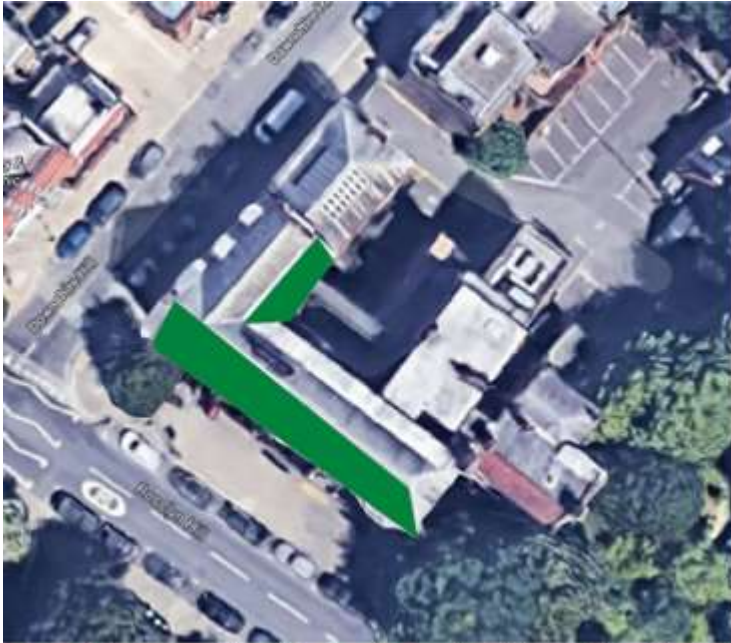
Figure 8 - Appropriate pitched roof areas for PV installation (if not listed)
