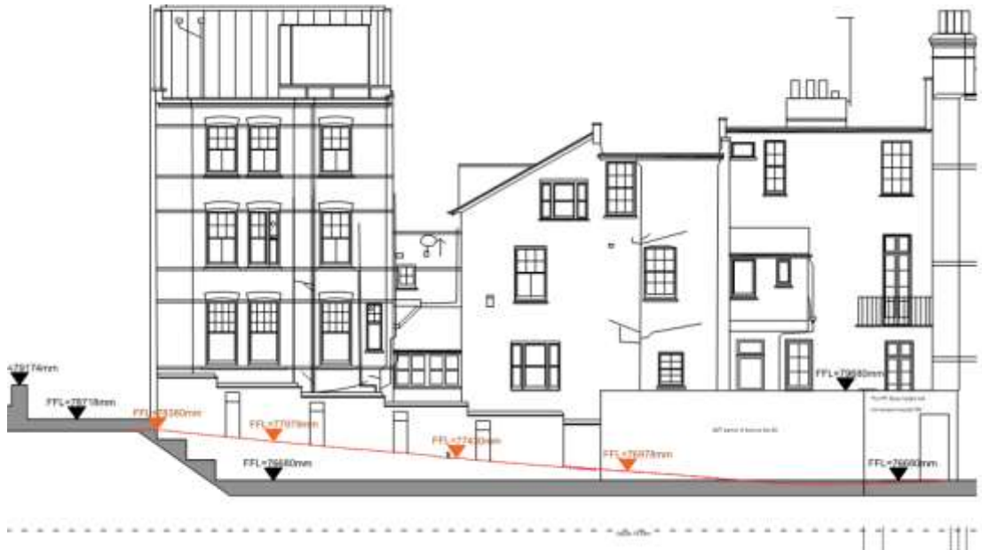
Figure 3 – acoustic barrier and rear of Downshire Hill properties (application drawings)
