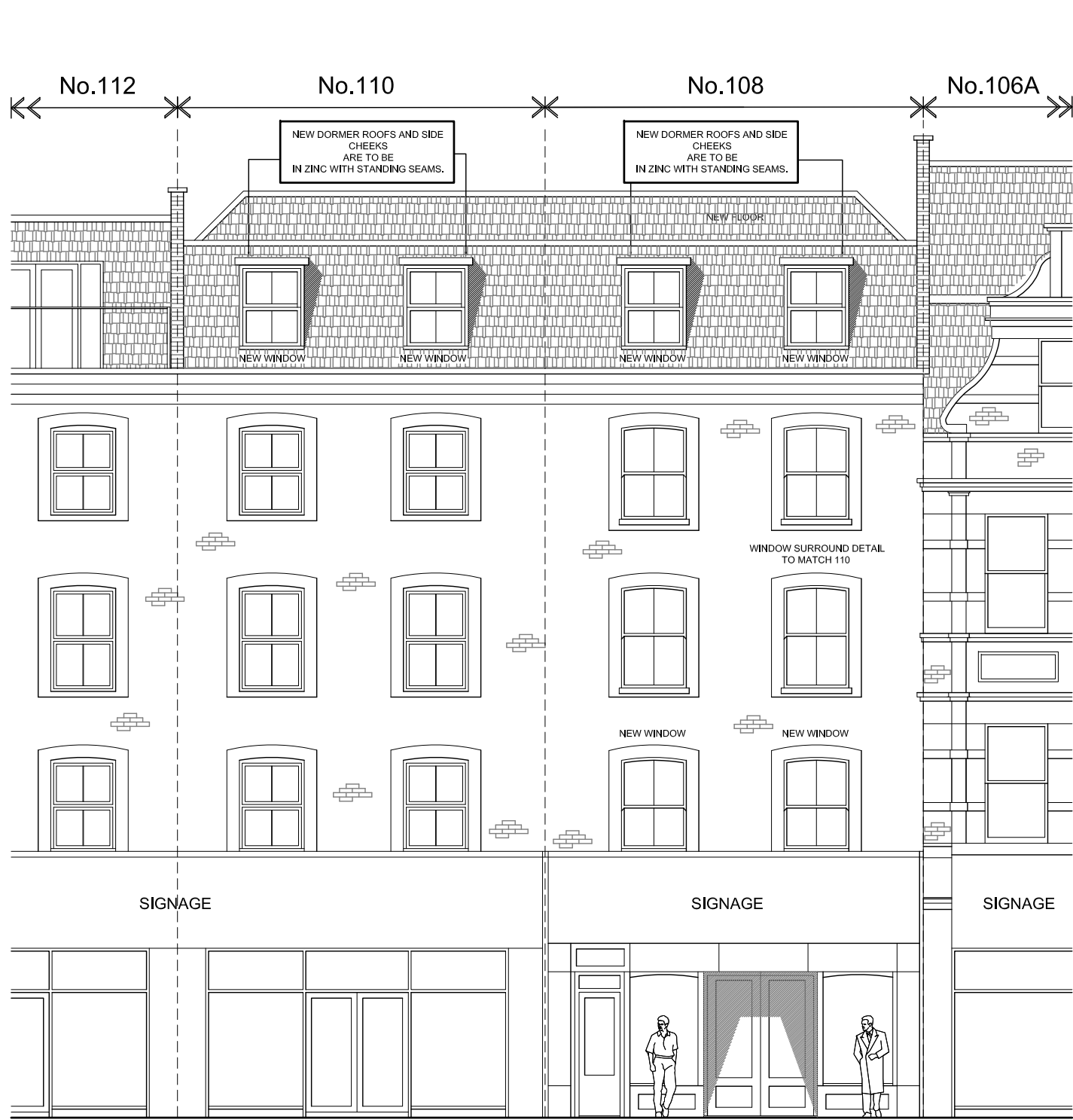
PROPOSED FRONT SOUTH WEST ELEVATION
