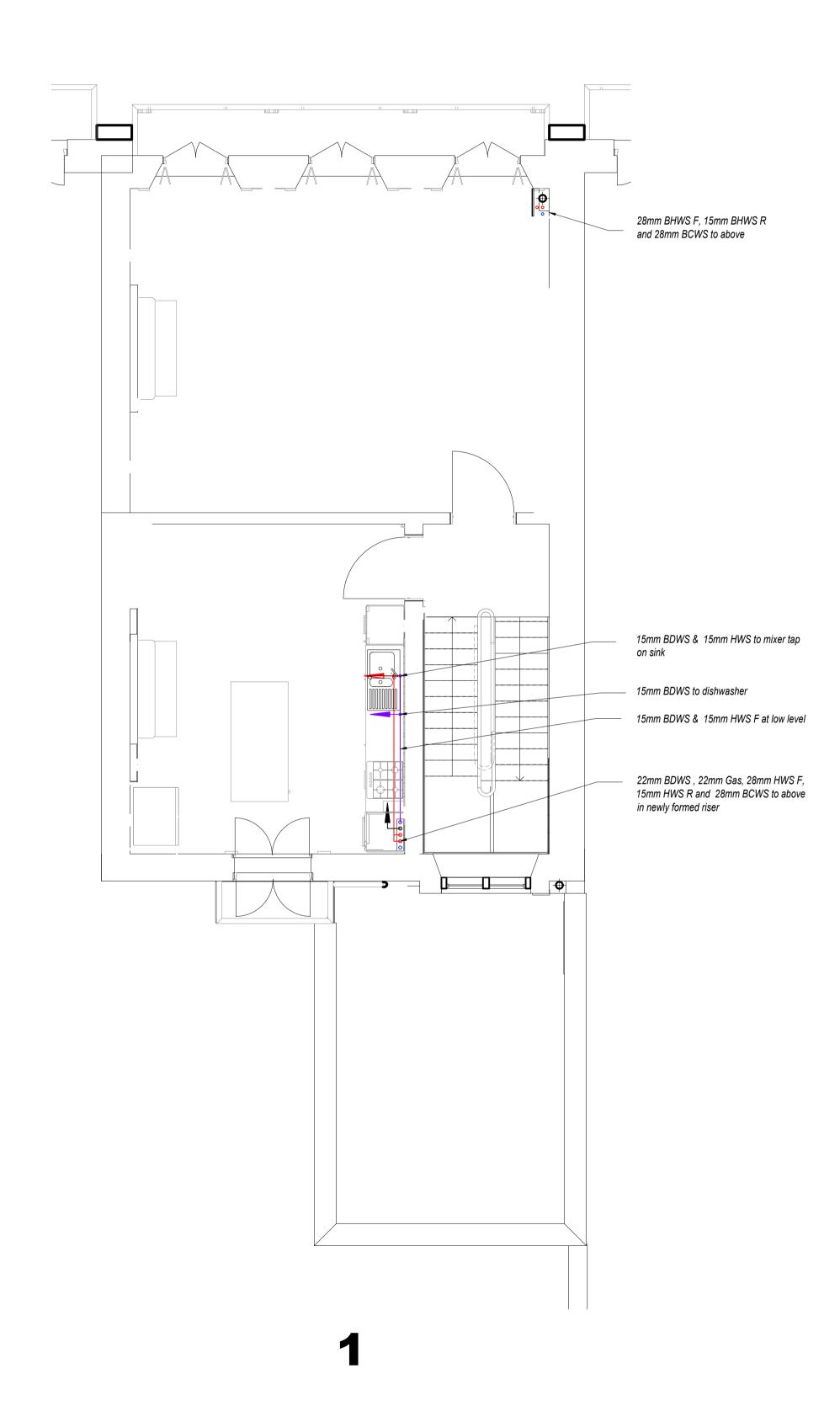
Note Each set of outlets to be fitted with PRV's on both hot and cold services.
