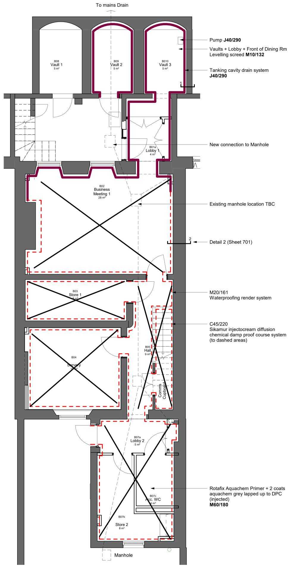
**B0 Waterproofing tanking** Scale 1:50
