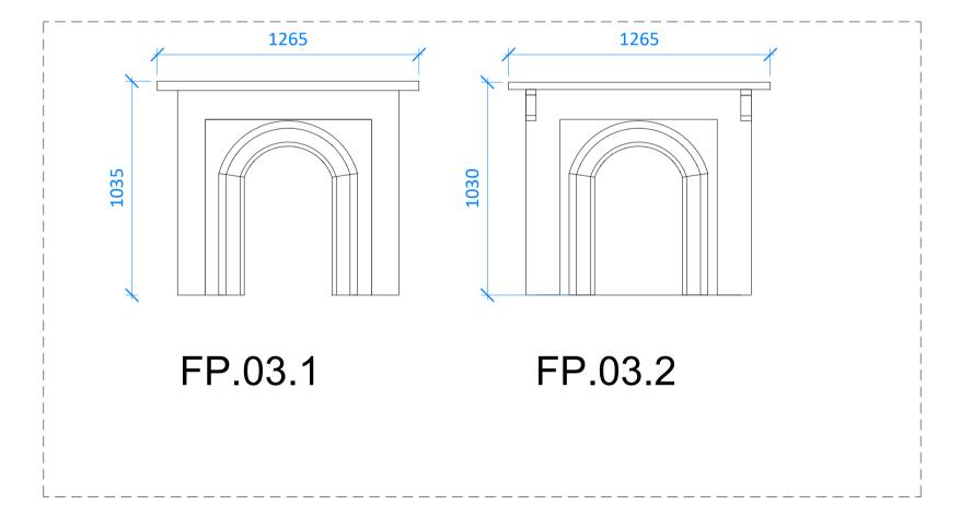
All dimensions to be verified on site by GENERAL CONTRACTOR prior to any work, setting out or shop drawings being prepared.
