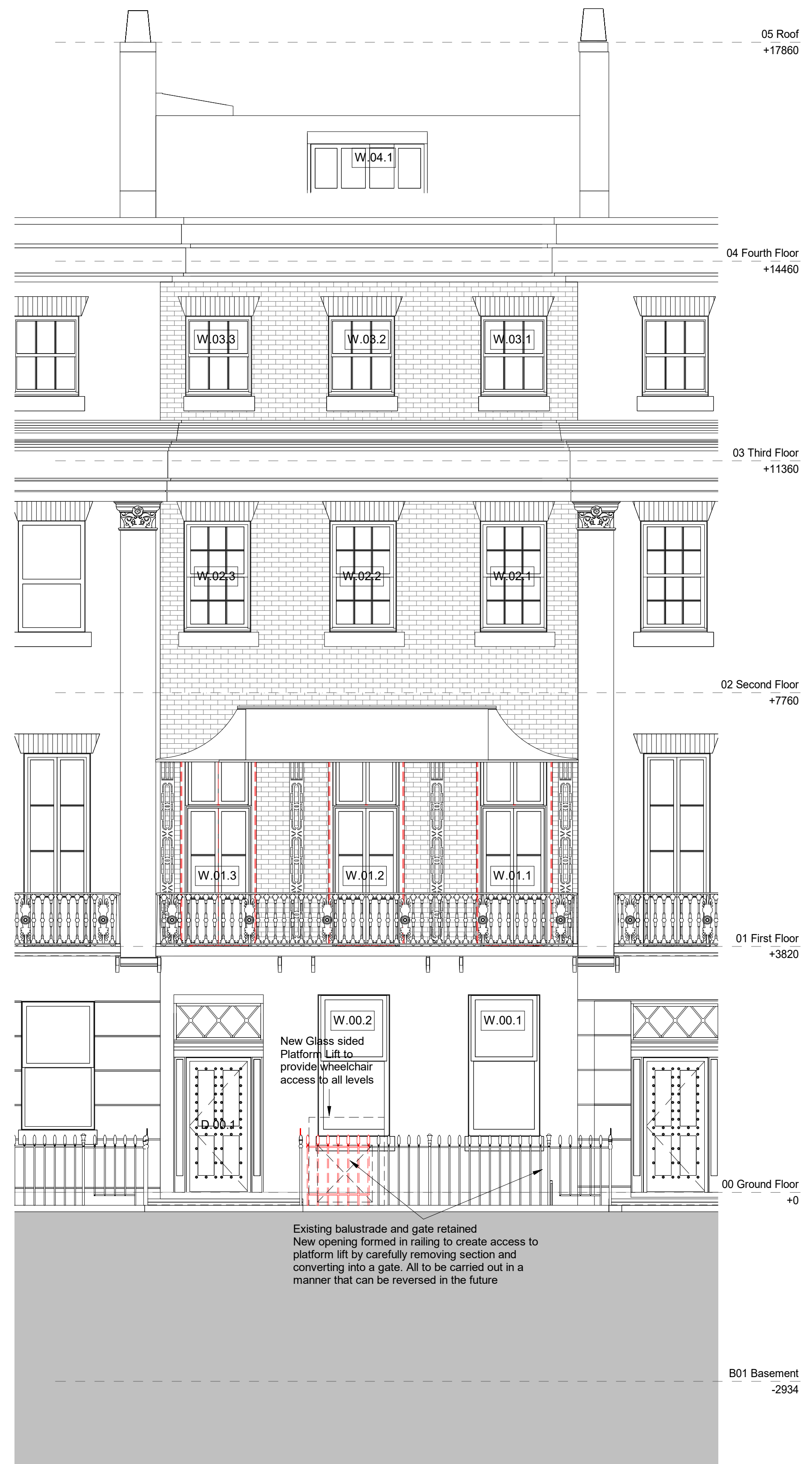
GA Proposed Front Elevation Demolition Scale 1 : 50
