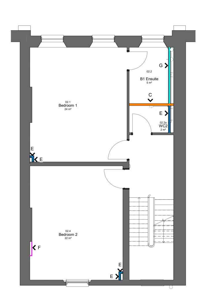
02 Proposed Second Floor Wall Types Plan Scale 1:50
