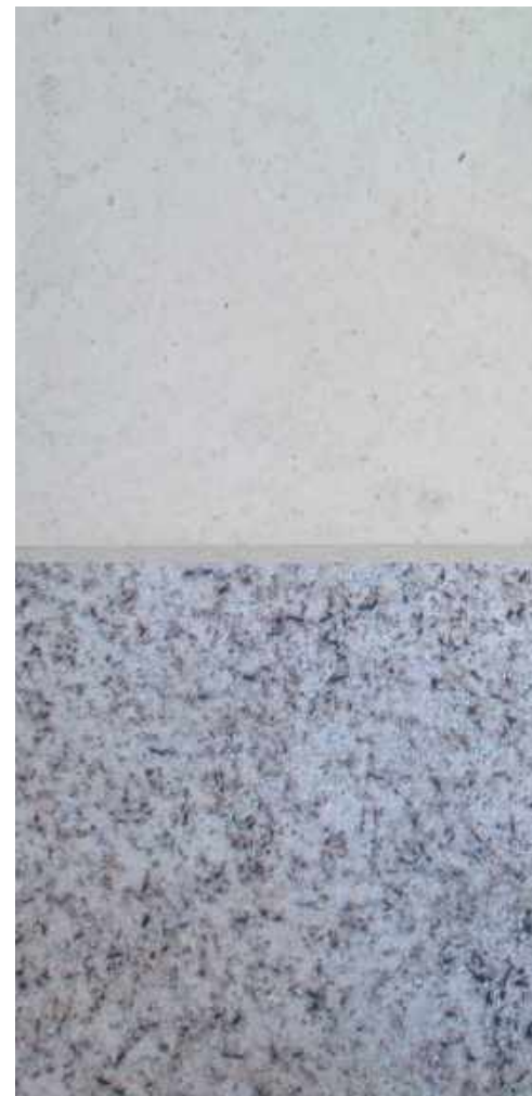
Moleanos Limestone (top) & Macieira Flamed Granite sample (bottom)
