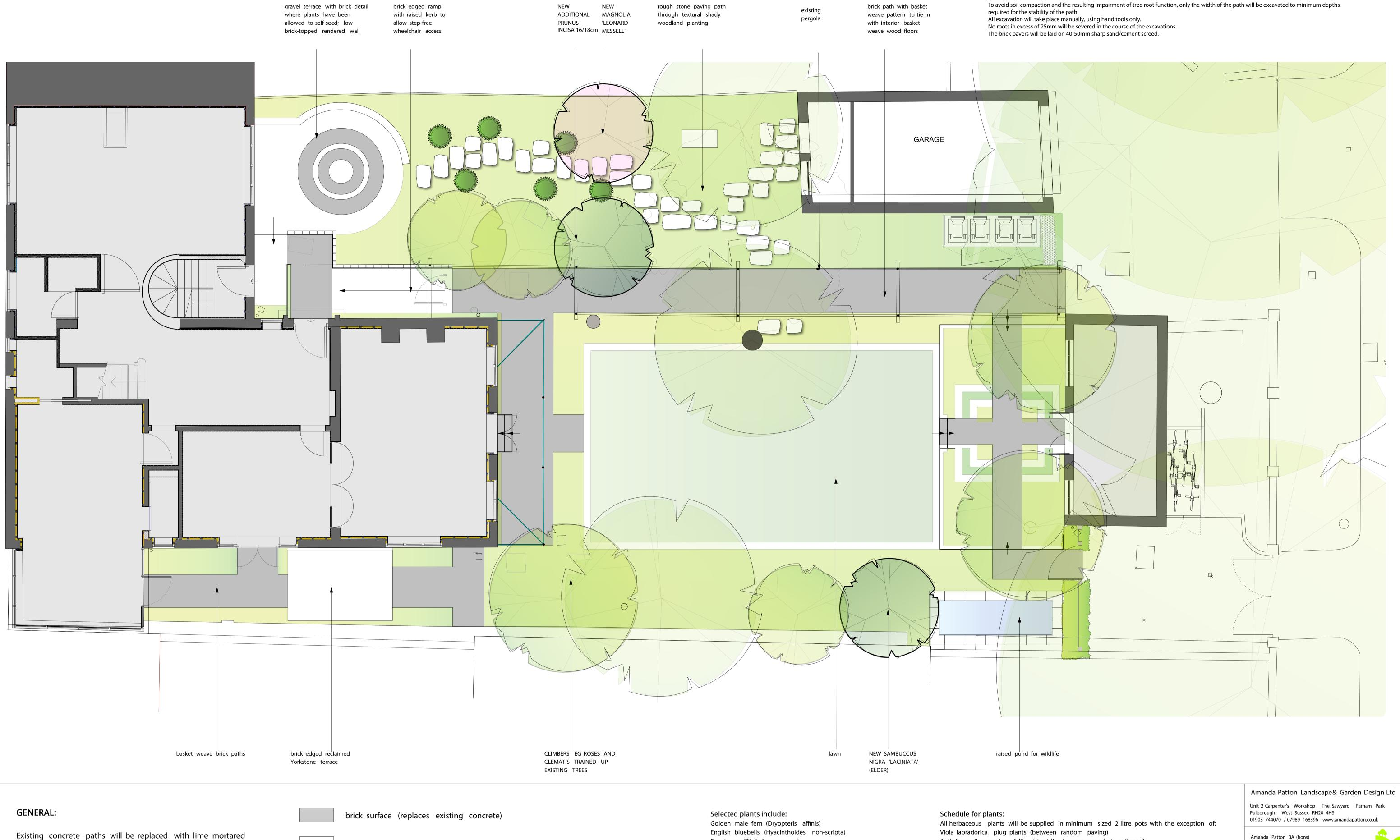
Existing concrete paths will be replaced with lime mortared brick paths in a basket weave pattern to match interior parquet wood floor.
