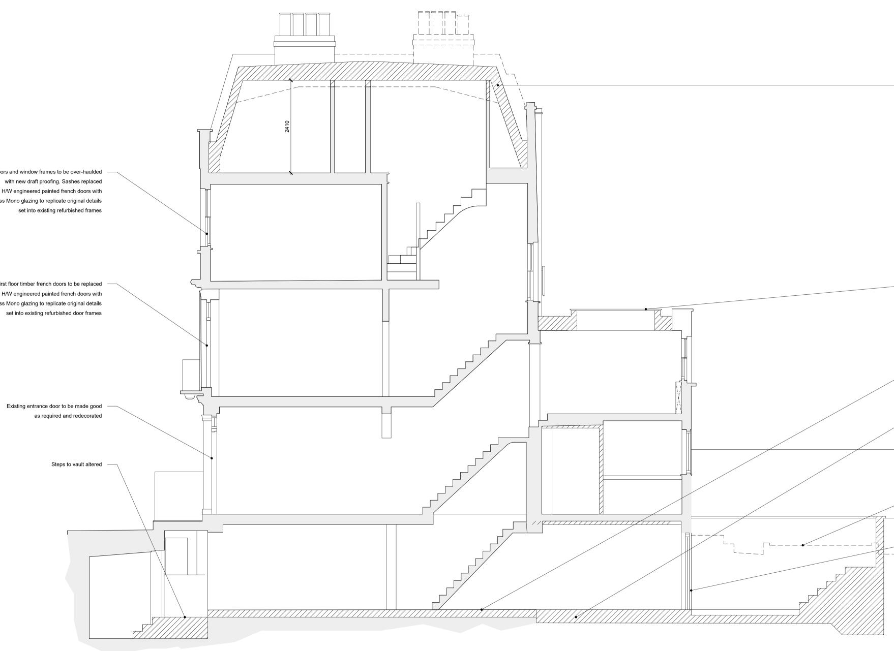
All existing doors and window frames to be over-haulded with new draft proofing. Sashes replaced with new H/W engineered painted french doors with Histoglass Mono glazing to replicate original details
