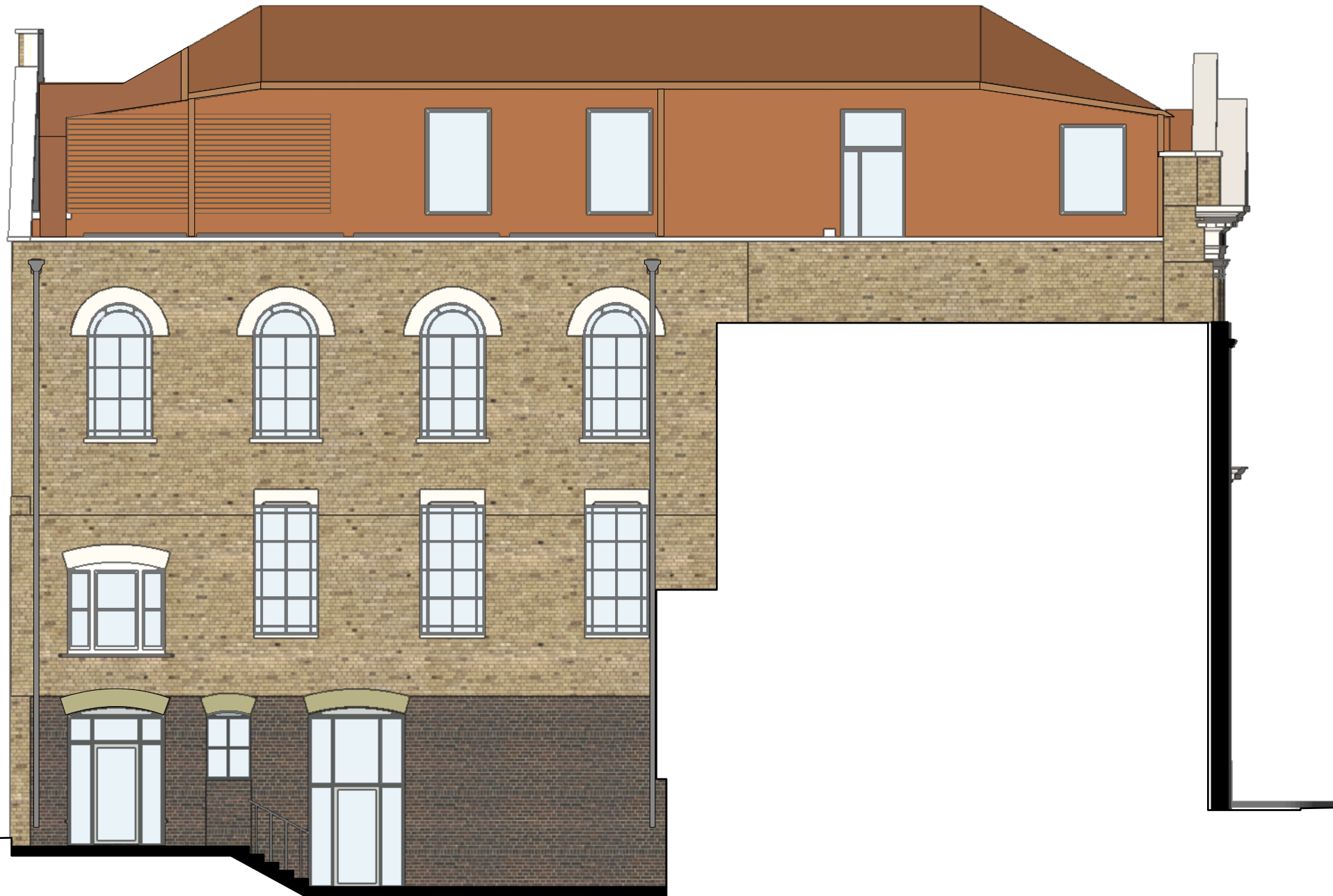
Proposed Side (East) Elevation Scale: 1:100
