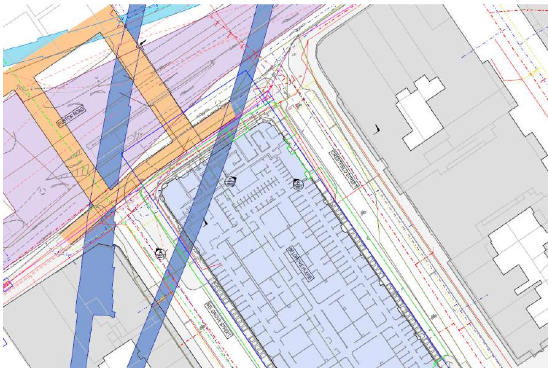
Figure 12 – Extract of site constraint plan indicating location of Piccadilly Line tunnels and Kings Cross station entrance tunnels
