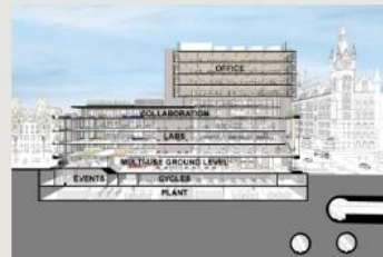
Cross section of Belgrove House showing the uses for each floor
