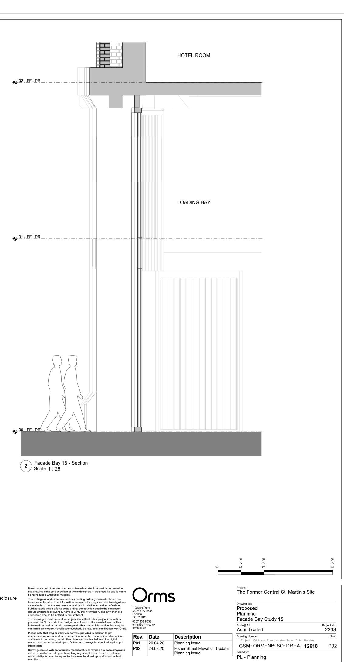
29 Metal cladding to plant enclosure 30. Timber louvres
