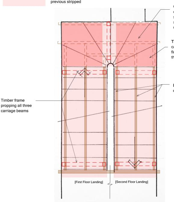
Once arrangement of carriage timber in winder section of stair known, strip finishes over full underside of stair.
