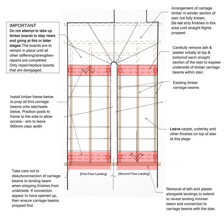
Plan of stair between first floor to second floor landings (not to sacle)
