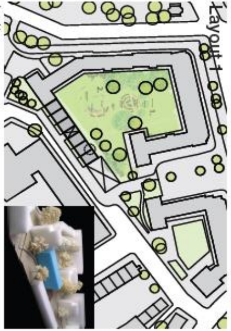
Layout 1 This is a three story terrace that follows the original pavement line of Chatham Street and then returns towards the space between Cowden and Crowndale Courts. The positioning of the terrace on the original pavement line allows for a small front garden to the terrace and the re-establishment of Chatham Street as a single lane, one-way street.
