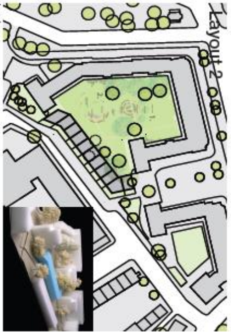
Layout 2 This proposal is a three story terrace that follows the original pavement line of Chatham Street and then returns towards the space between Cowden and Crowndale Courts. The positioning of the terrace on the original pavement line allows for a small front garden to the terrace and the re-establishment of Chatham Street as a single lane, one-way street.
