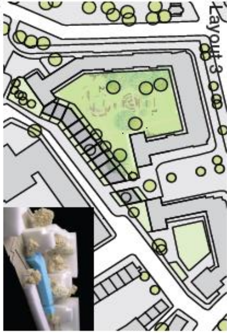
Layout 3 This proposal is also for a three story terrace that follows the original pavement of Chatham Street until meeting the line of Crowndale Court. A section is reserved to form an entrance line between Crowden and Crowndale Courts. This positioning of the terrace on the original pavement line allows for a small front garden area to the terrace and the re-establishment of Chatham Street as a single lane, one-way street.
