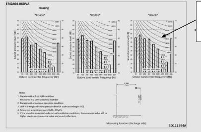
Noise data for Daikin model ERGA08DVA full duty heating mode = overall 49dBA. Noise data is in terms of free field overall dBA & linear dB octave band sound pressure level values at 1m in front of the unit.
