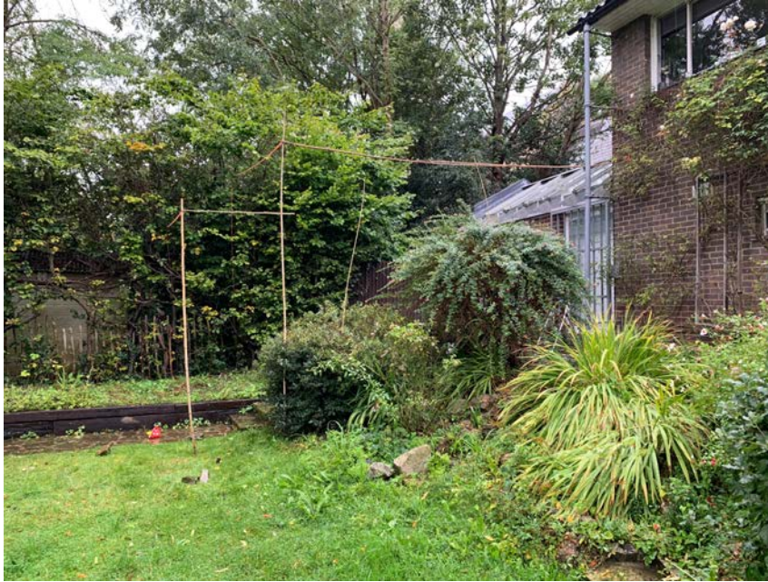
1:1 scale test marking the height of proposed extension. Subsequently the height is reduced to only 2 m above the upper terrace level.
