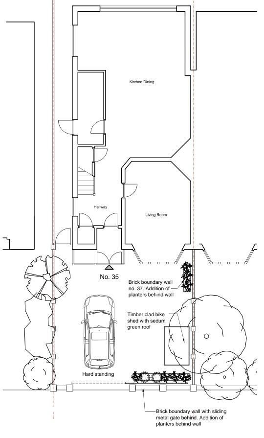
Revisions A 07.08.20 Bike shed amended to timber clad with sedum roof. **EXISTING & PROPOSED PLANS** 35 Swains Lane Holly Lodge Estate **GROUND FLOOR & FRONT GARDEN** Drawing No Scale This drawing and all the designs herein are the sole property of HAT and may not be used without written authorisation.
