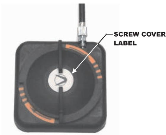
Once the knob is inserted, fasten the closing screw, insert the sheath and turn the knob to the UNRELEASED position. In this position, only the orange part of the label must be seen with the drawn black arrows.
