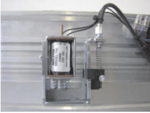
Insert the compression spring and insert the metal cable inside the special release anchor, then lock it with the screw clamp. Adjust the cable tension so to give the spring a light pre-load.
