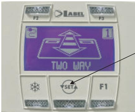
By pushing the central button **YSETA** select the automatic door work mode. Each time a button is pressed, it switches from a work program to the next one.
