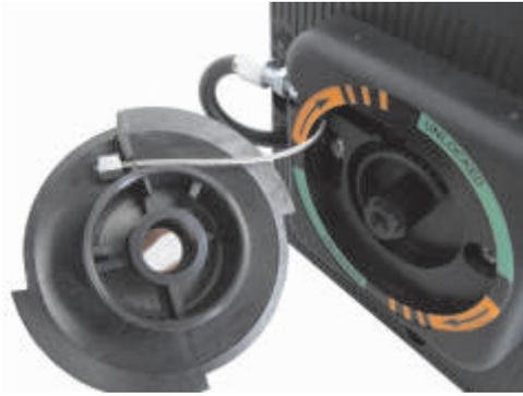
Fasten the base of the release knob to the side panel using 2 self-threading screws, making the bend pipe enter the hole made in the side panel.
