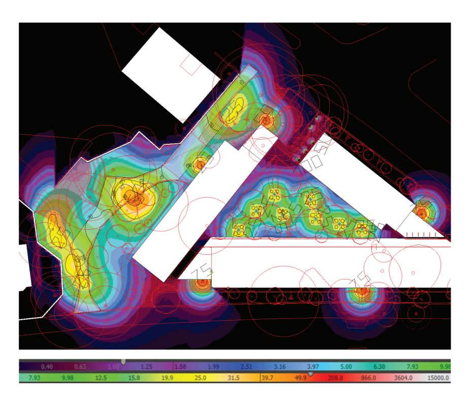
Site plan showing lux levels to the pedestrian walkway and courtyard with proposed lighting design
