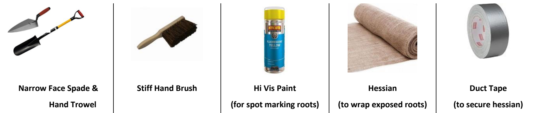
Fig 4 – Advised tools for any hand digging activity
