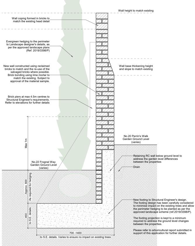
Proposed Elevation and Section Detail  $(\mathbf{1})$
