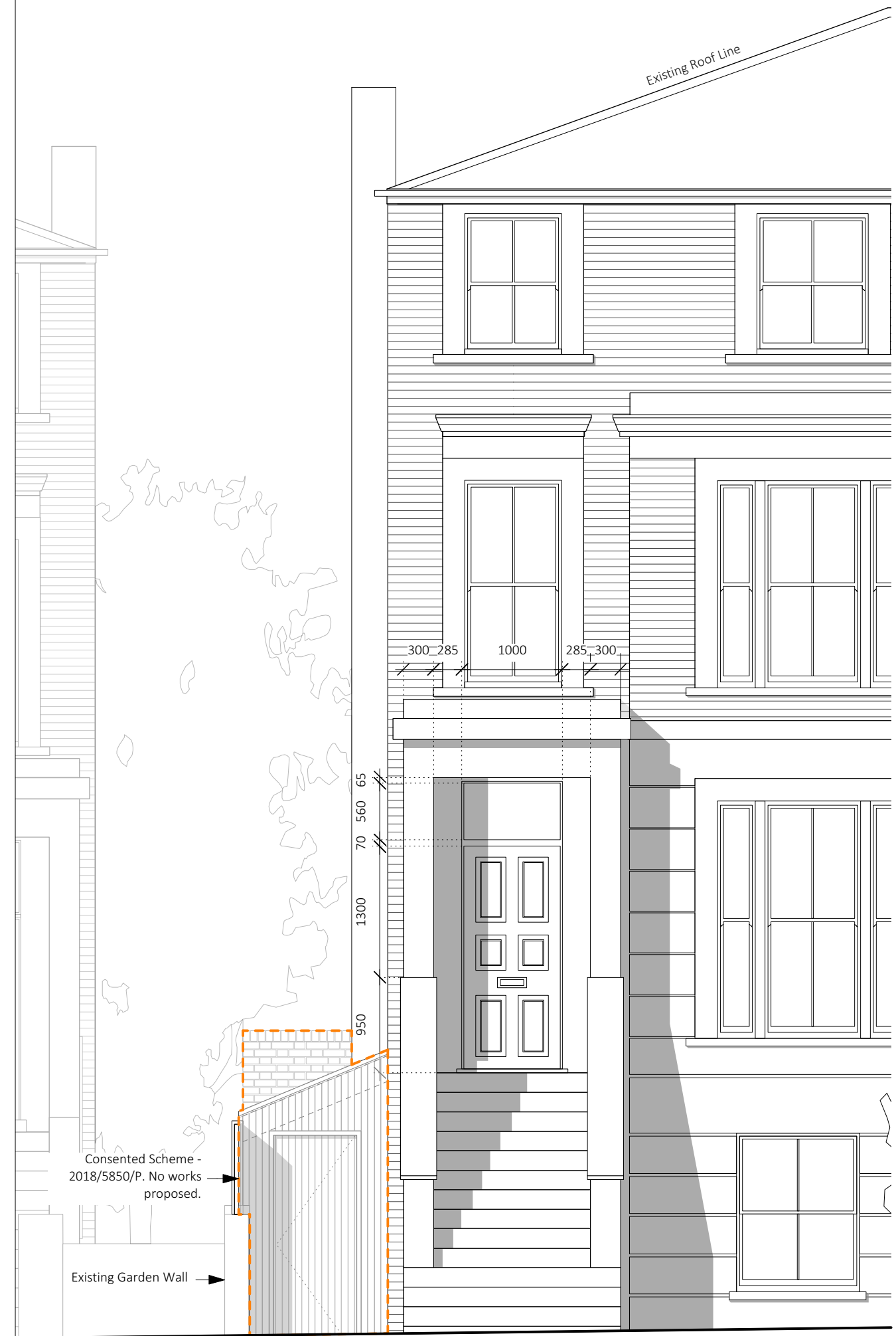
Existing - Front Elevation
