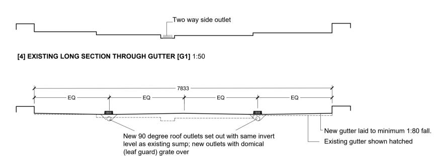
[5] PROPOSED LONG SECTION THROUGH GUTTER [G1] 1:50
