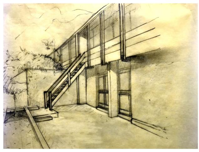
**SKETCHED IMPRESSION ONLY** SHOWING PROPOSED TIMBER STAIRCASE CONNECTING UPPER FLOOR EXISTING BALCONY AND LOWER FLOOR ALLOWING DIRECT ACCESS FROM UPPER LEVEL TO GARDEN LEVEL WITHOUT HAVING TO GO THROUGH THE BEDROOMS:
